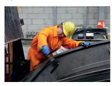
Then continue with the remaining small sides (longitudal joint sides), also starting from the middle and going towards the corners. Again take care that you equably distribute the material along the groove and check again that all sections are sufficiently clipped in.
