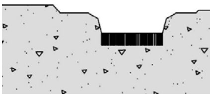
Groove section after removal of damaged profile
