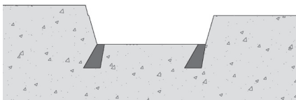
Groove section after removal of damaged profile
