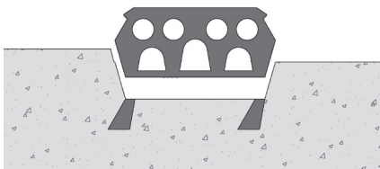
Repair profile to be inserted and glued in
