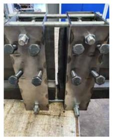
After applying the cyberbond, bring the profile ends together by tightening the screws quickly from the bottom up! Tighten the Screws until the adhesive comes out between the gaskets ends. The gluing needs the pressure for best bonding results. You can remove the assembly aid after 2 hours. The final bonding strength is reached after 24 hours. Now the start seal is ready to use and can be installed and fixed properly into the metal holding construction holding rail.
