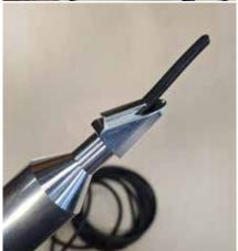
The cord is inserted from the back of the tool until a piece peeks out at the front.
